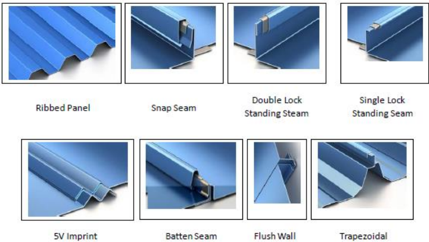
Figure 4: Types of roll forming profiles
