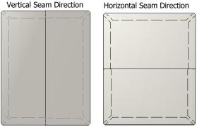
NOTE: Retrofit covers are beneficial when a standard one piece cover cannot be slid over the feature being flashed. The cover seam can either be oriented vertically or horizontally.
