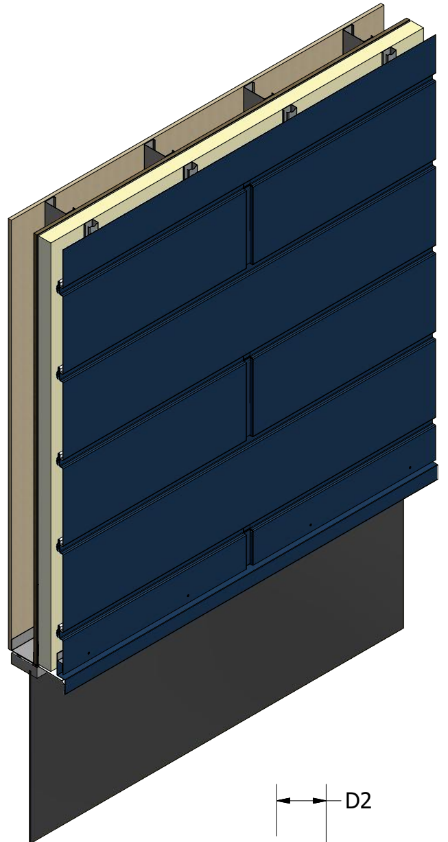
Head Flashing (field fabricated from color matched flat stock)
