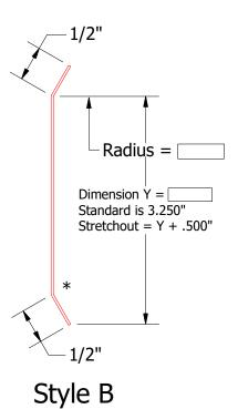
Concave: Convex: Material 24 ga 55% Al-Zn alloy coated Alum steel with acrylic coating Finish: Color: Trim Length: Number of Pieces:
