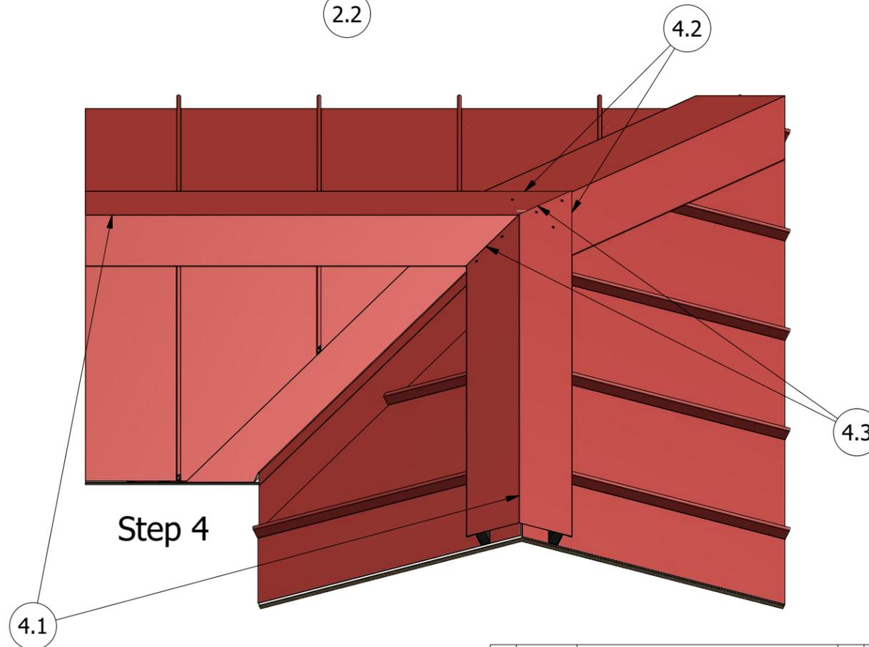
**Step 1.1** Install Valley Pan with Joggle Cleats, Butyl Tape and Appropriate Fasteners.
