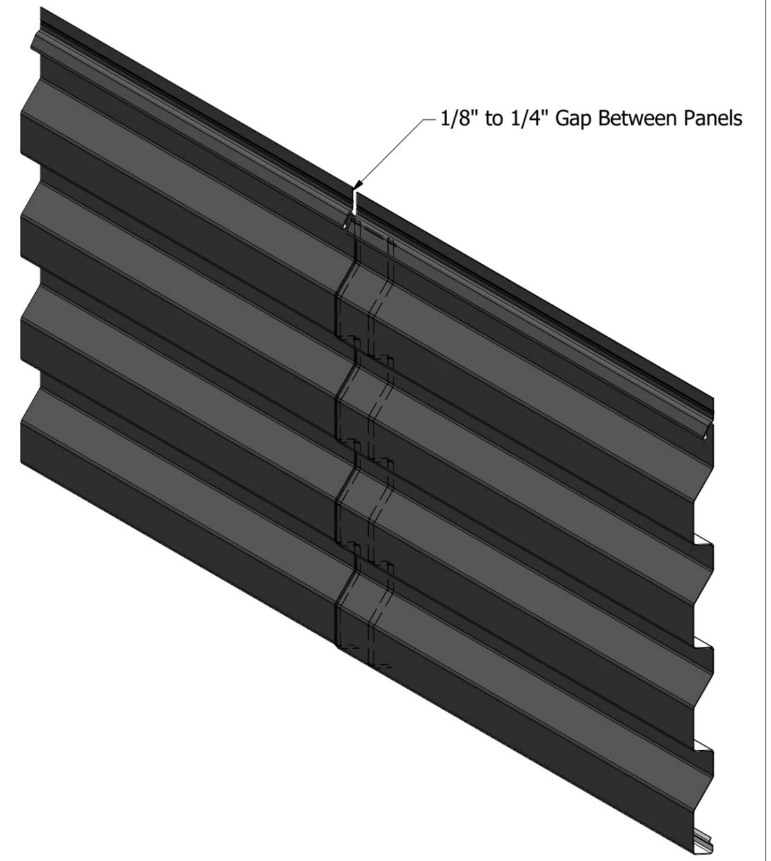
**Note:** Factory Pre Notching is Available (direction of panel is required).
