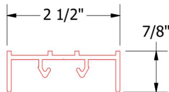
MAY902 - Receiver Extrusion for Flush Transition Cover
