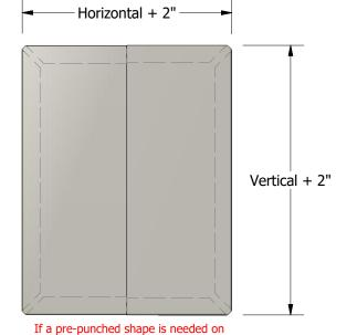
NOTE: Retrofit covers are beneficial when a standard one piece cover cannot be slid over the feature being flashed. The cover seam can either be oriented vertically (as shown) or horizontally.
