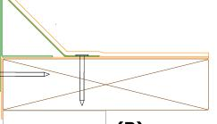
(B) Install Strip-in Membrane over top of 24 GA Cant per Membrane Manufacturer's Directions.
