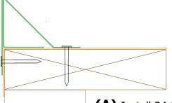
(A) Install 24 GA Cant with 3" Leveling Angle onto Substrate and Roof Membrane.
