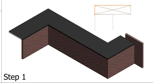
2) Locate and position Notched Cant at any scupper locations. Install a 3" Leveling Angle 1 ½" inside each side of the notched Cant. With the Cant plumb and tight to top of the Leveling Angle, secure it to the blocking with provided 1 1/2" ring shank nails. Install one nail through each slotted hole at 12" O.C. front and top (See Detail A). Position scupper in the notched Cant and secure by nailing through the pre-punched holes in the Roof Flange.
