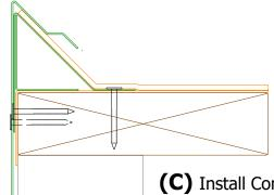
(C) Install Continuous Spring Cleat on top of Strip-in Membrane and 24 GA Cant.
