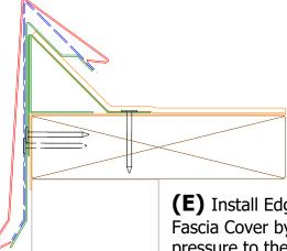
(E) Install Edge Lok 3 Fascia Cover by applying pressure to the top.
