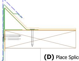
(D) Place Splice Plates at ends of Inside/Outside Miters and at the ends of the Straight Fascia Covers.
