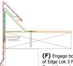
**(F)** Engage both Hems of Edge Lok 3 Fascia Cover then release to snap in place.
