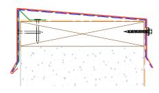
Secure back of Coping Cover with #9 x 1 1/2" Screws through pre-punched slots at 17" O.C.
