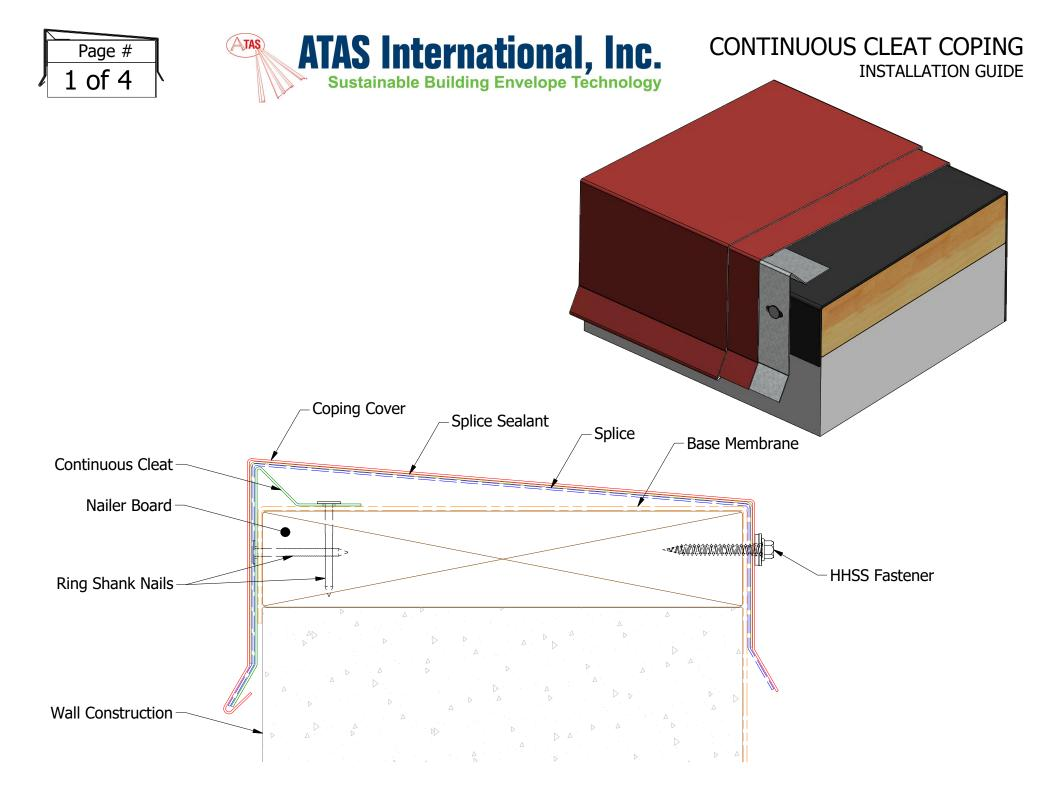
**Step 1.1** Check to make sure wood nailer and waterproofing membrane are installed correctly.
