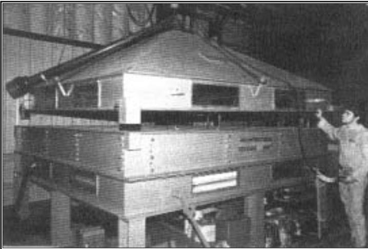
**Typical chamber for testing uplift pressure.**
