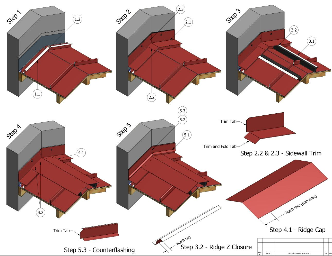
Step 1.1 Install Sidewall Z Closures on to Roof Panels with appropriate accessories.
